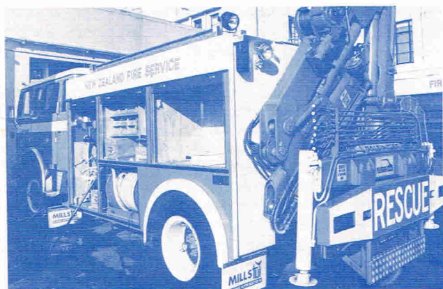
Rescue Unit with Hydraulic Rear Crane—Unit is also fitted out with air compressor, for supplying hand tools.
